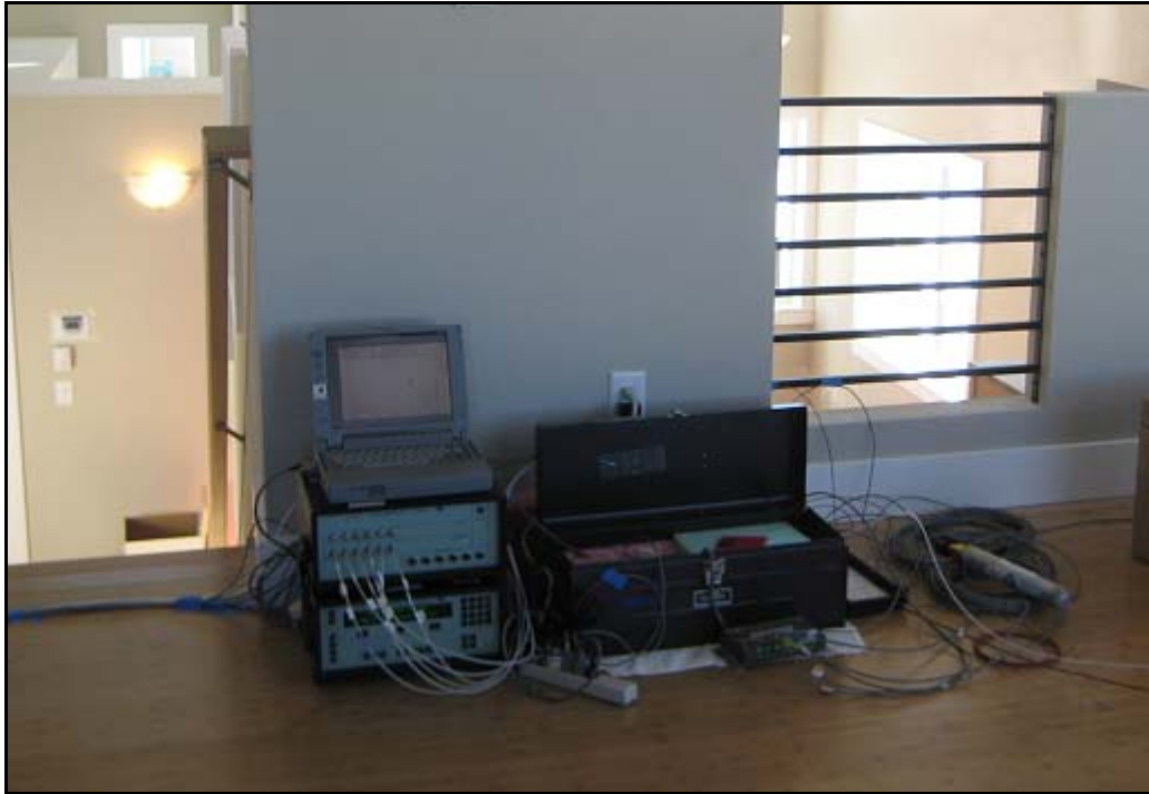
Figure 19: Photo of tracer gas set-up in unit 1.
